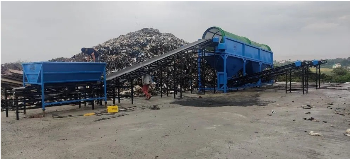
Figure 26: Trommel screen used for waste segregation in India
