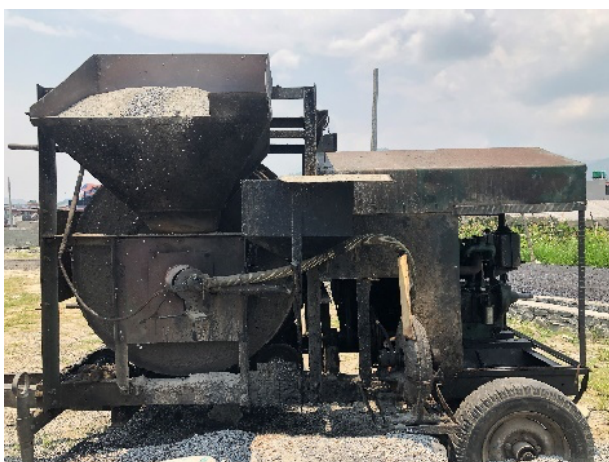
Figure 10: Spot-mix on a construction site, June 2023
